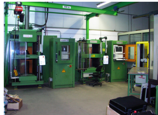
Retrofit of hydraulic and electrical Reicherter sprint testing machines (300 and 25kN)
