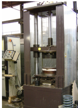
Retrofit of hydraulic Wolpert testing machine with X-Y-table for measuring side loads and side rate of railway springs
