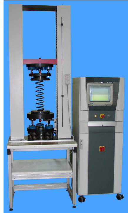
CADIS testing machine 81870 (25 / 50kN) for testing automotive springs. Measuring eccentricity of piercing points, side loads and bending moment
