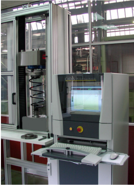
CADIS testing machine 81870 (25 / 50kN) for testing automotive springs. Measuring eccentricity of piercing points, side loads and bending moment
