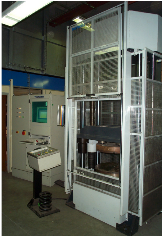
Spring testing machine 81822 (300kN) for railway springs with motorized X-Y-table for measuring side movement, side load and side rate of springs. Three axis, simultaneous closed loop control for travel and load
