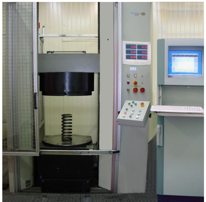
UTS-spring testing machine 600kN with CADIS control system (retrofit)
